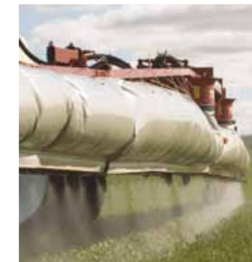
TWIN FORCE A curtain of air from under the boom carries the spray droplets to the target reducing drift and increasing coverage.
