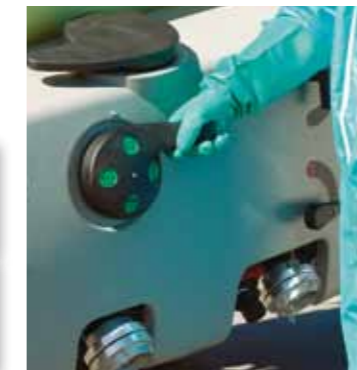
SmartValves Filling and cleaning is controlled by two colour coded valves for easy operation.
